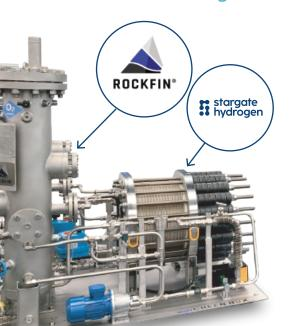
**Rockfin** built customized hydrogen production systems based on Stargate's pressurised alkaline stacks.
