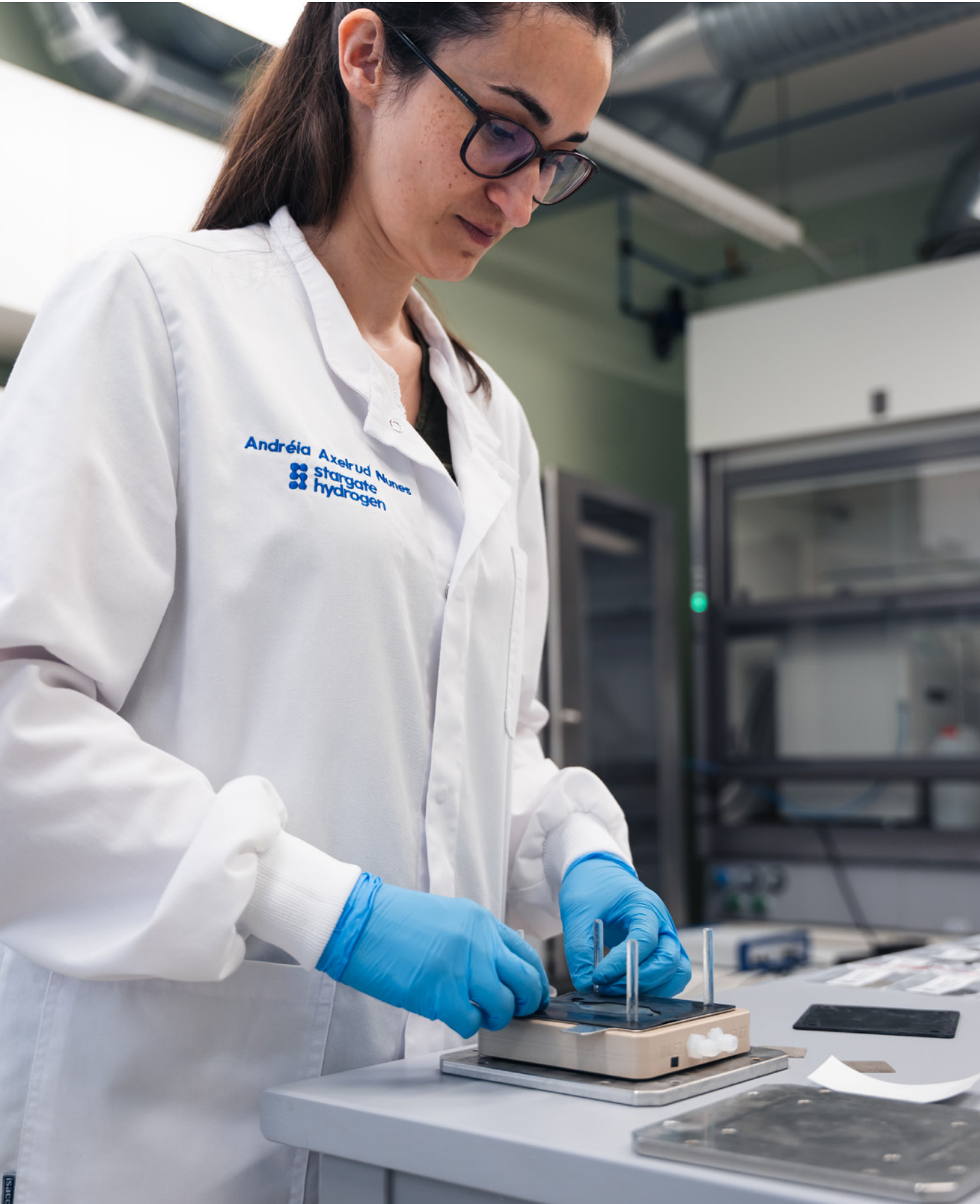
Preparing an electrolysis cell for electrochemical testing at Stargate's research laboratory.
