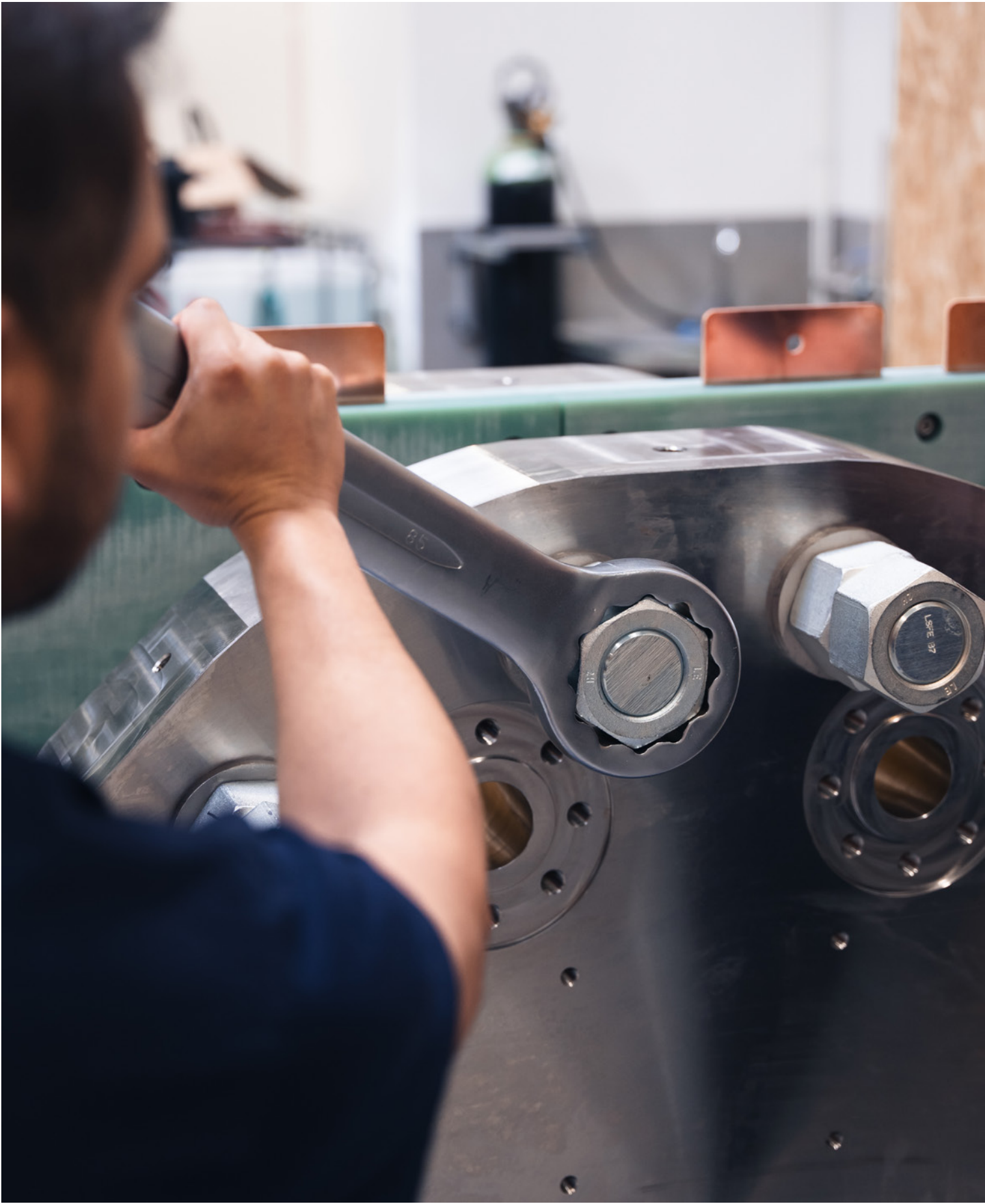
Tightening the bolts on an electrolyser stack at Stargate's production facility.
