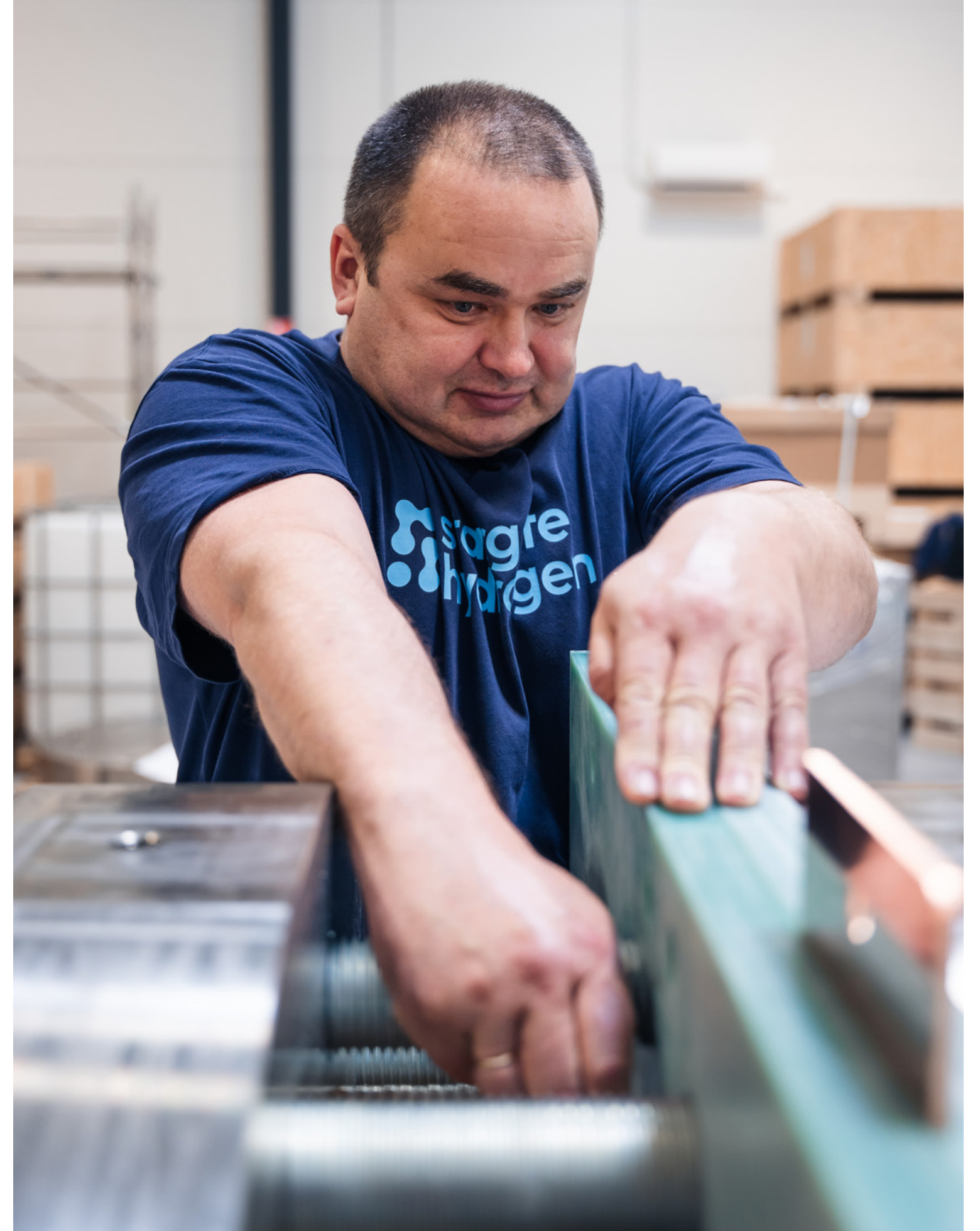
A Stargate employee puts the finishing touches on an electrolyser stack.
