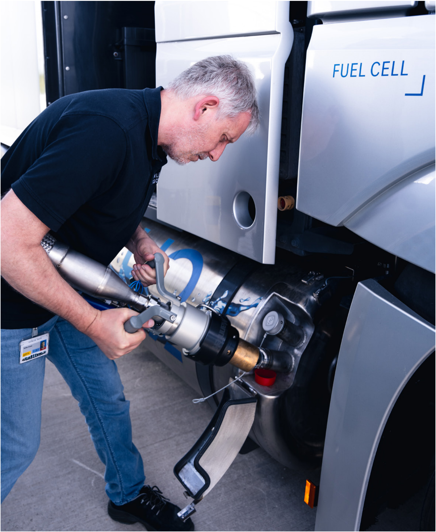
Refilling the GenH2 Truck with sLH2 liquid hydrogen.
